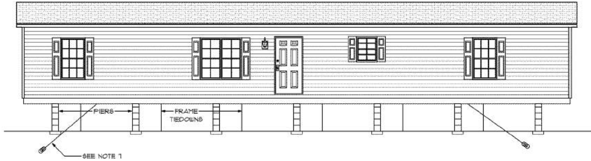
TYPICAL SIDE ELEVATION SHOWING TIEDOWN SPACINGS
